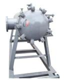
200 PSIG, 12" 150# connections Carbon steel, 316 SS internals Holds 19 x 80" cartridges
