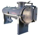
1480 PSIG, 12" 600# connections Carbon steel, 304L SS internals Holds 12 x 80" cartridges
